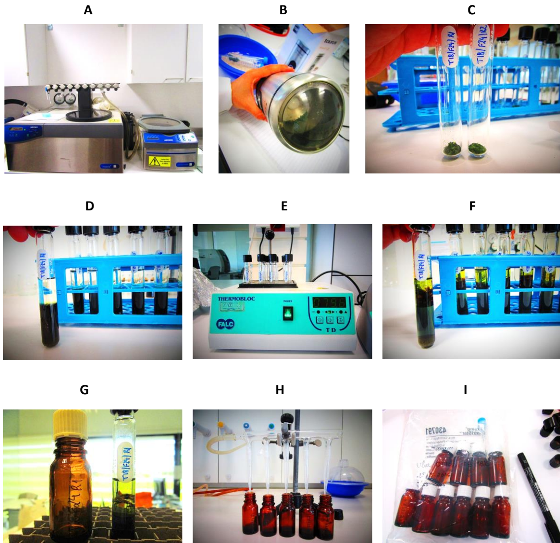
Fig. 8 - Direct Transesterification process. A: lyophilization, B: grinding; C: samples for extraction; D: sample with methanol and acetyl chloride; E: heating (80 °C); F: complete transesterification with phase separation (upper phase contains n-hexane and FAME, lower phase contains other metabolites, water and methanol); G: FAME phase collection to amber vial; H: evaporation of n-hexane under nitrogen stream; I: sample vials storage.
