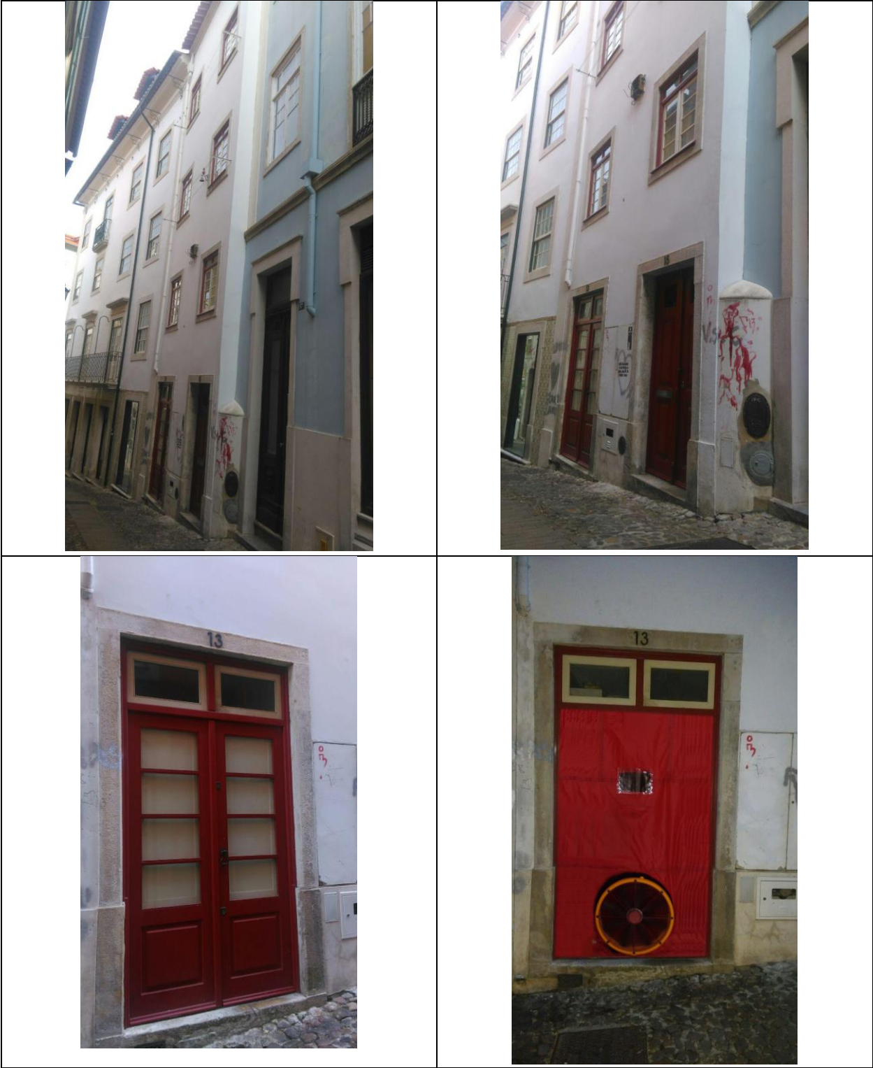
Figure 160: Interior and exterior properties of windows of the apartment. Also the procedures of BDT in the fourth case study
