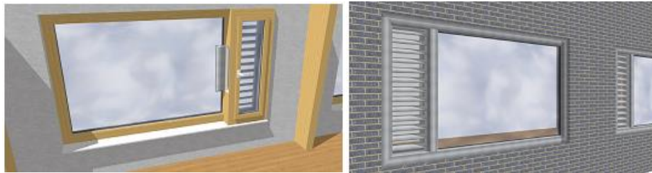
Figure 111: Combination of air-vent with the window structure [230]
