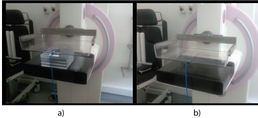
Figure 5.5: Experimental configurations. a) To measure the ESD, the PMMA phantom has to be included and for b) the measurement of K_{air} , the IC remains in the same position even with the absence of the phantom.
