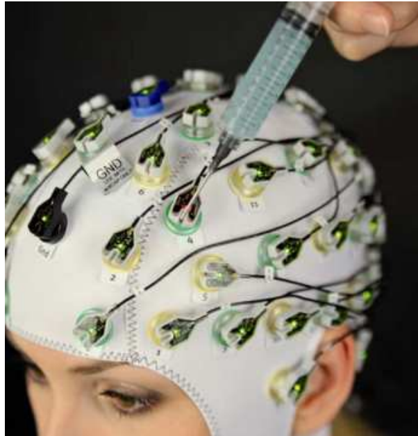
Figure 4.4 – Representation of Brain Products® actiCAP with 64 possible active electrodes, from BrainProducts (Brain Products GmbH, 2016).
