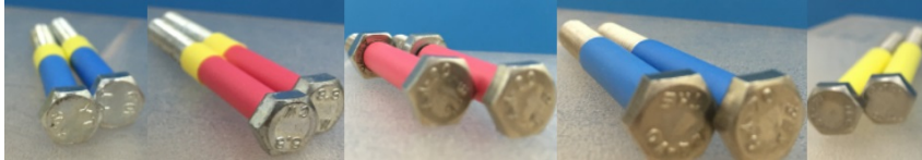
Figure 4.9: First electrodes used to water tests: YT 10,9, ZP 8,8, A4 80, A4 70, A2 70, respectively.
