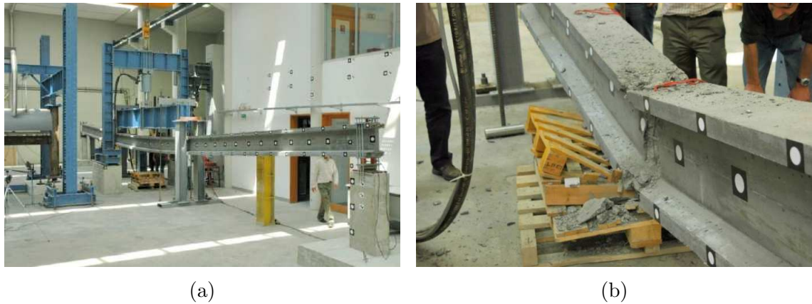
Figure 4.9: Experimental test of HSC girder: (a) test set-up; and (b) failure (Fernandes, 2005).
