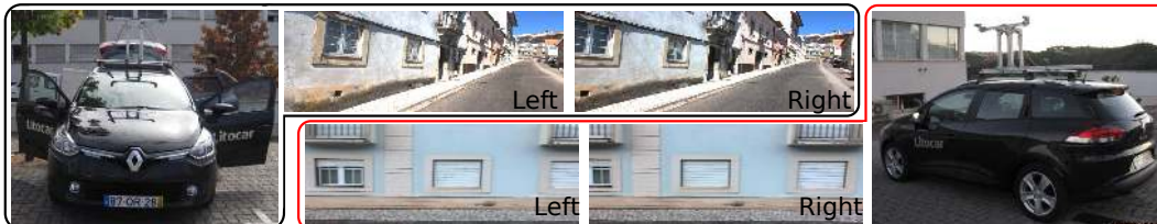
(b) Cameras mounted on a car and respective acquired stereo pair
