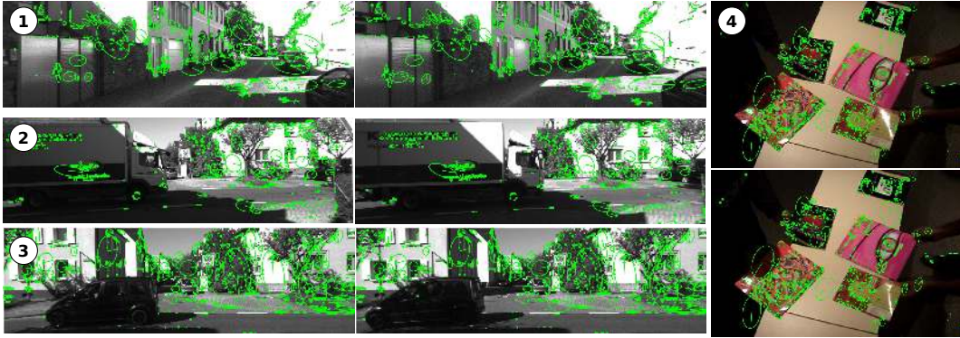
Figure 4.9: Image pairs with the extracted ACs for 4 different scenarios: 1 - normal motion, 2 - dominant dynamic foreground, 3 - static camera/pure rotation, and 4 - four motions besides the camera motion. Examples 1 to 3 are from the KITTI dataset [42,43] and Example 4 is from the Hopkins dataset [131]. \pi Match is applied to each scenario and the results are shown in Figures 4.10 and 4.11.
