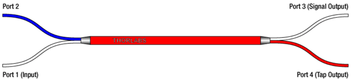
Figure 3.9 Graphical representation of the fibre optic coupler's ports. Reproduced from [33].
