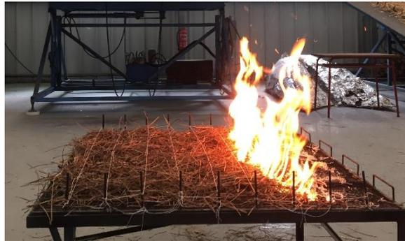
Figure 3.9: Determination of the basic rate of spread  $R_0$  in a fuel bed of pine needles.
