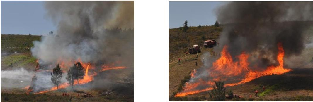
Figure 3.14: Digital photos in the experimental tests in the field of junction fires with formation of firewhirls.
