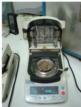
Figure 3.3: Moisture analyser A&D ML50.
