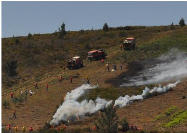
Figure 3.13: Ignition of the two fire fronts along their entire length with the pyrotechnic system in the field.
