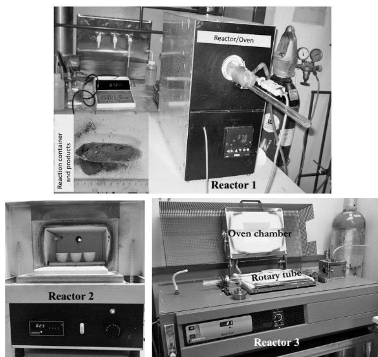
Figure 12 – Reactors used for the solid/solid reaction of magnesium silicates with ammonium salts, at ÅA (taken from Nduguagu (2012)).
