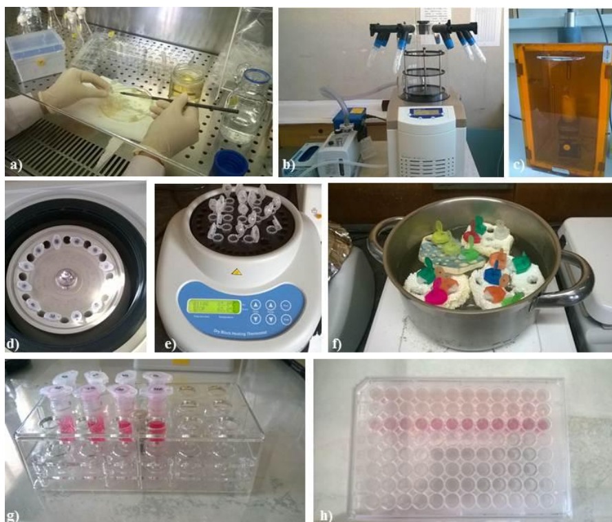
Figure 25 – Chitin quantification: a) mycelia collection; b) lyophilization; c) sonication; d) centrifugation; e) evaporation; incubation in boiling water; samples at room temperature; samples inoculated in 96 multi-well plate.
