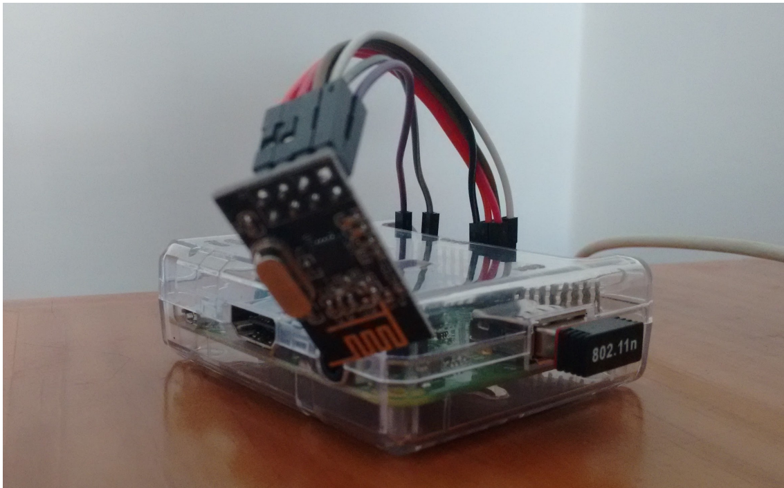
(a) Schematic version of the gateway. It is constituted by a Raspberry Pi and a NRF24L01+ radio transceiver.
