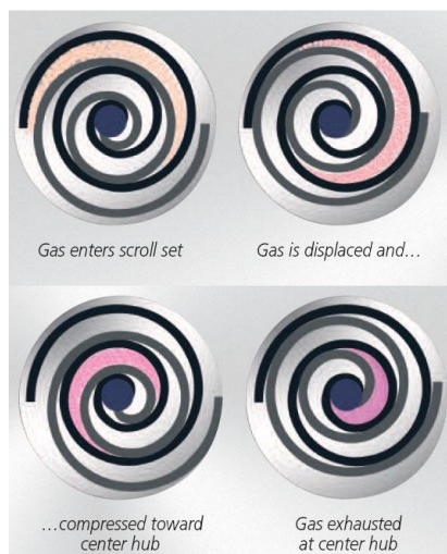
(a) Scroll Pump function diagram [1].
