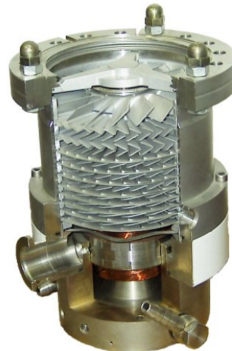
(b) A cutaway view of a turbomolecular high vacuum pump. 11
