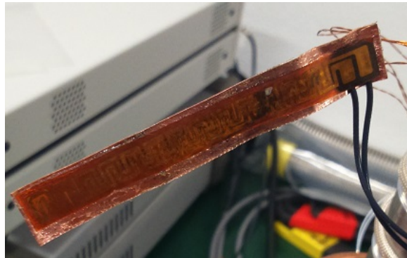
Fig. 4.9 Foil heater glued to a cooper foil
