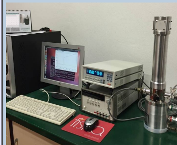
Figure 2: Closed cycle helium cryostat and temperature control module of the AC susceptometer
