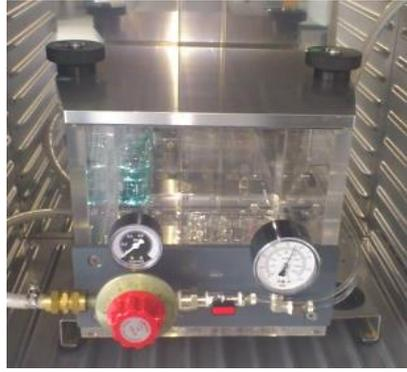
**Figure 13** – Pressure chamber. Humidified pressure chamber, equipped with a regulator to ensure +70 mmHg, placed inside an oven at 37°C.
