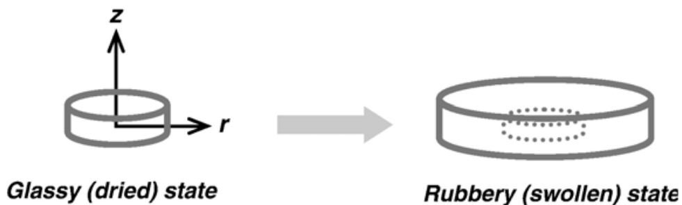
Figure 1.12 – Illustration of the change in size of a hydrogel in a dry and swollen state. [28]
