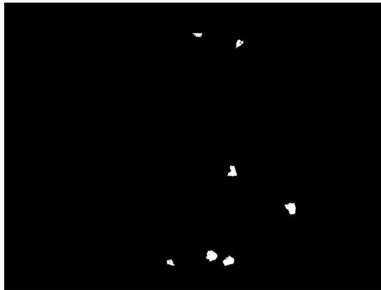
Figure 4.15: Binary image of the detected laser mark candidates using Laser Mark Segmentation.
