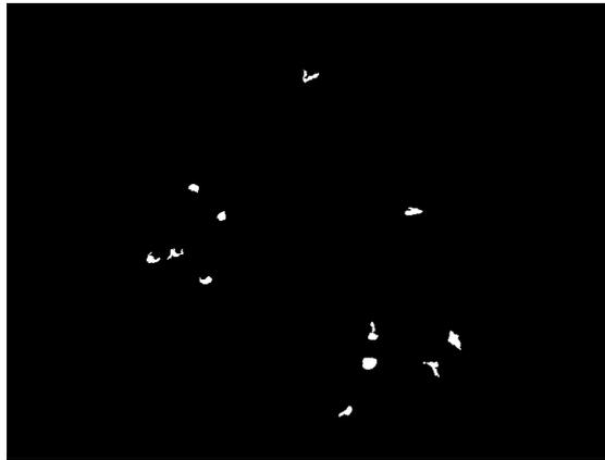
Figure 4.14: Binary image of the detected laser mark candidates using Frangi Vesselness Filter.
