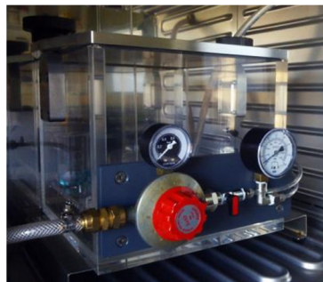
Figure 11– Image depicting the pressure chamber. Humidified pressure chamber equipped with a regulator to ensure + 70 mmHg, and placed at 37°C.
