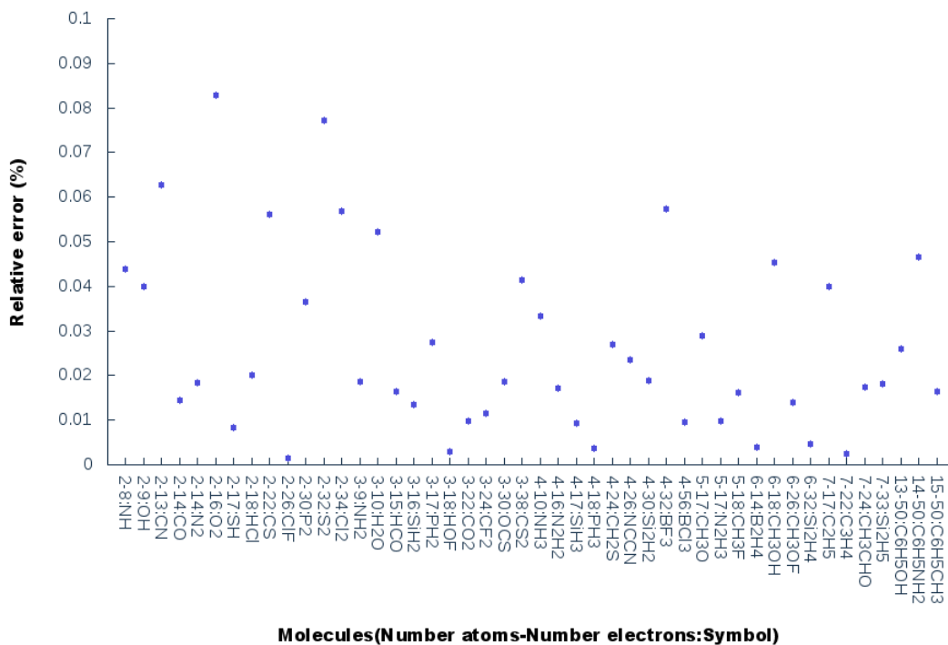
Fig. 6.8 Error value of the GGA_X_SSB_SW + GGA_C_SOGGA11_X for each molecule sorted by number of atoms and number of electrons.
