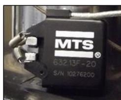
**Figure NB.2.** MTS extensometer.
