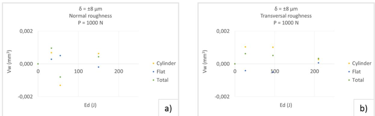
**Figure PB.7.** Evolution of wear volume with dissipated energy for the 2 components (cylinder and flat) and for the total amount (sum of both). For a displacement amplitude of  $\pm 8 \mu\text{m}$ , a normal force of 1000N and a) Normal roughness and b) Transversal roughness.
