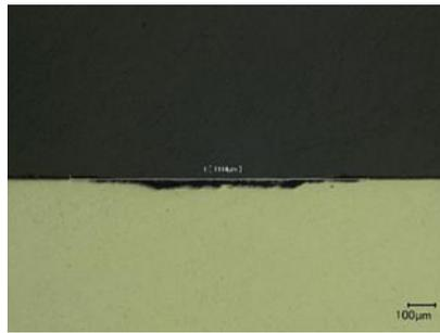
**Figure 3.23.** Image of a transversal wear scar taken by Keyence microscope with an amplification of 300x. Test conditions: flat with normal roughness subjected to 600 N of normal force, a displacement amplitude of  $\pm 40 \mu\text{m}$  and 50.000 cycles.
