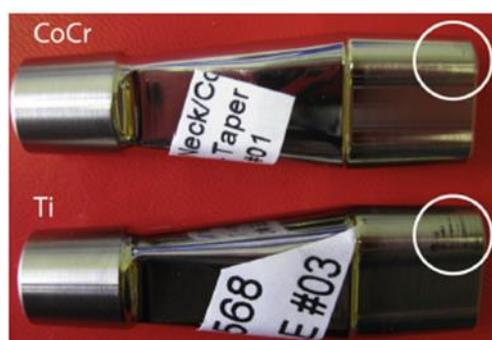
**Figure 1.6.** H-Max neck adapters after mechanical testing. In the laterodistal area of Ti neck adapters slight scratches could be observed (bottom). No surface damages at the Co-Cr neck adapters were seen (top) [13].
