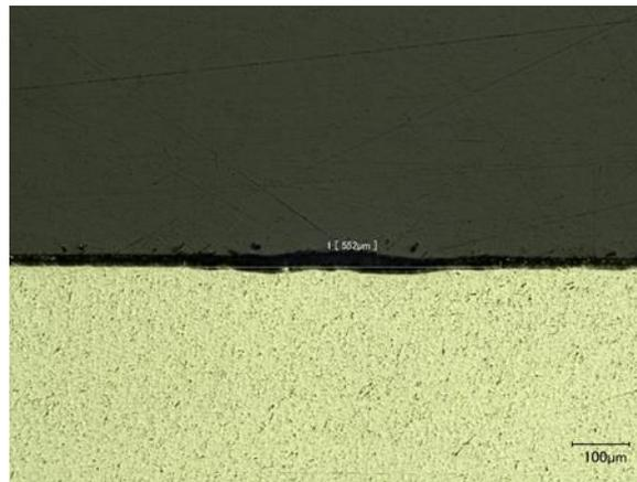
**Figure 2.13.** Image of a transversal wear scar taken by Keyence microscope with an amplification of 300x
