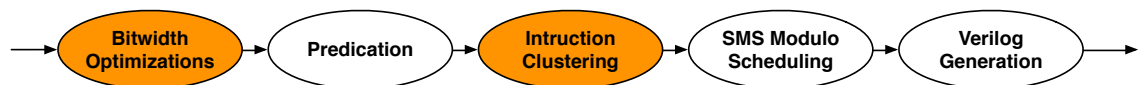
Figure 5.36: Sequence of SOpenCL backend code transformations and optimizations. Highlighted are the optimization steps of particular interest to LDPC decoding.
