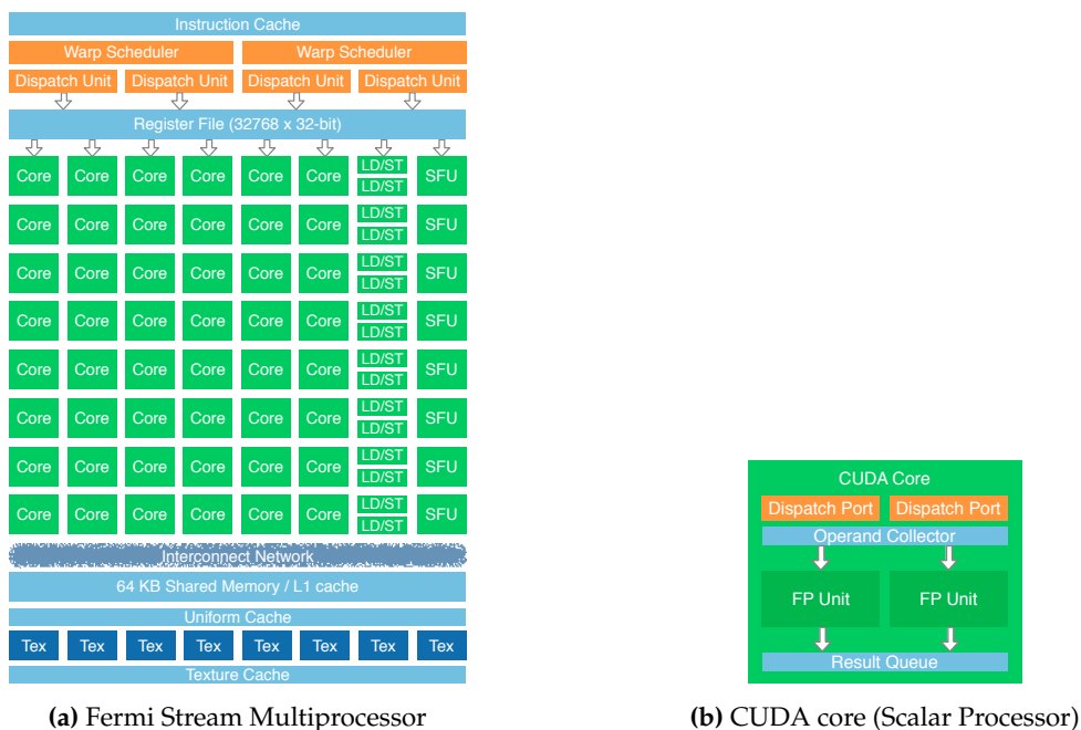
Figure 4.4: SIMT GPU SM and CUDA core in detail: a) Fermi SM and b) CUDA core or SP.
