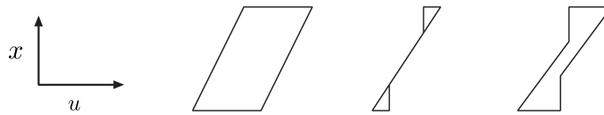
Figure 3.45: Typical patterns of a sticky valve.
