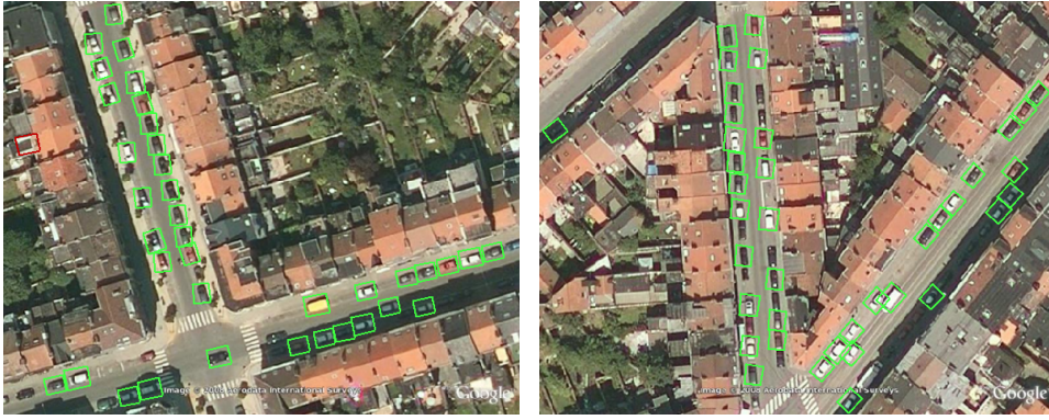
Figure 6.4: Example detections and estimated poses in the Google Earth dataset. In this dataset, an object’s pose is determined by the angle of rotation on the image plane, illustrated as a rotated bounding box. Best viewed in color.
