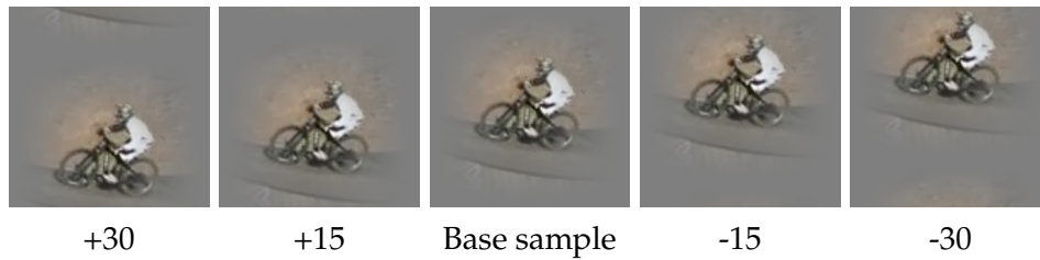
Figure 4.2: Examples of vertical cyclic shifts of a base sample. Our Fourier domain formulation allows us to train a tracker with all possible cyclic shifts of a base sample, both vertical and horizontal, without iterating them explicitly. Artifacts from the wrapped-around edges can be seen (top of the left-most image), but are mitigated by the cosine window and padding.
