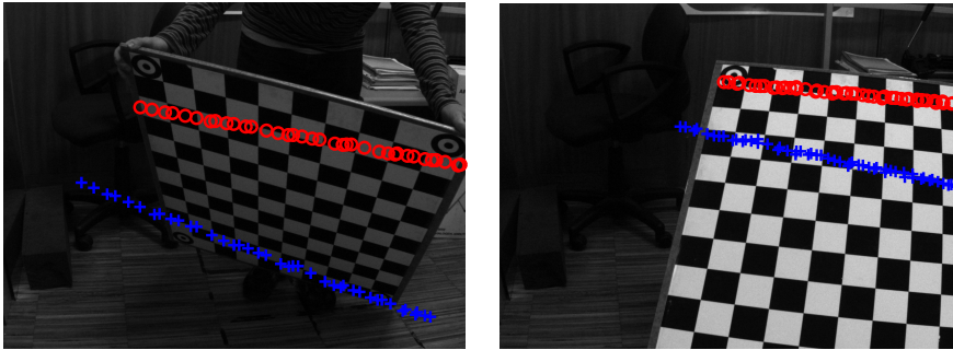
Figure 3.9: Projection of the LRF points into the images using the extrinsic calibration results obtained from 5 sampled planes with our method (circles) and Zhang's algorithm (crosses).
