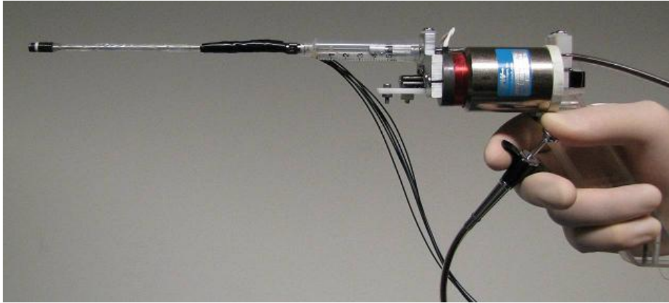
Figure 2.7: The hand-held robotic device for mitral valve repair surgery developed at the Harvard Biorobotics lab. (source: [Yuen et al., 2009]).
