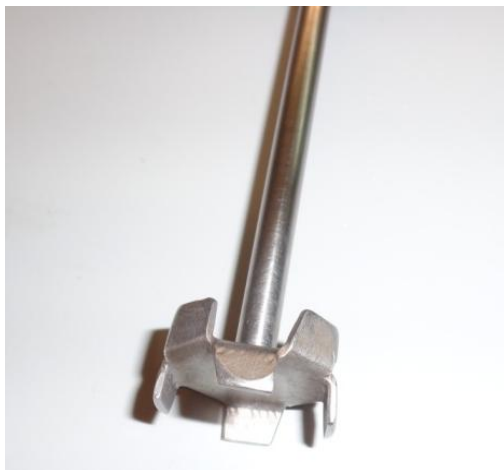
Figure 11 - Propeller shape stirrer.
