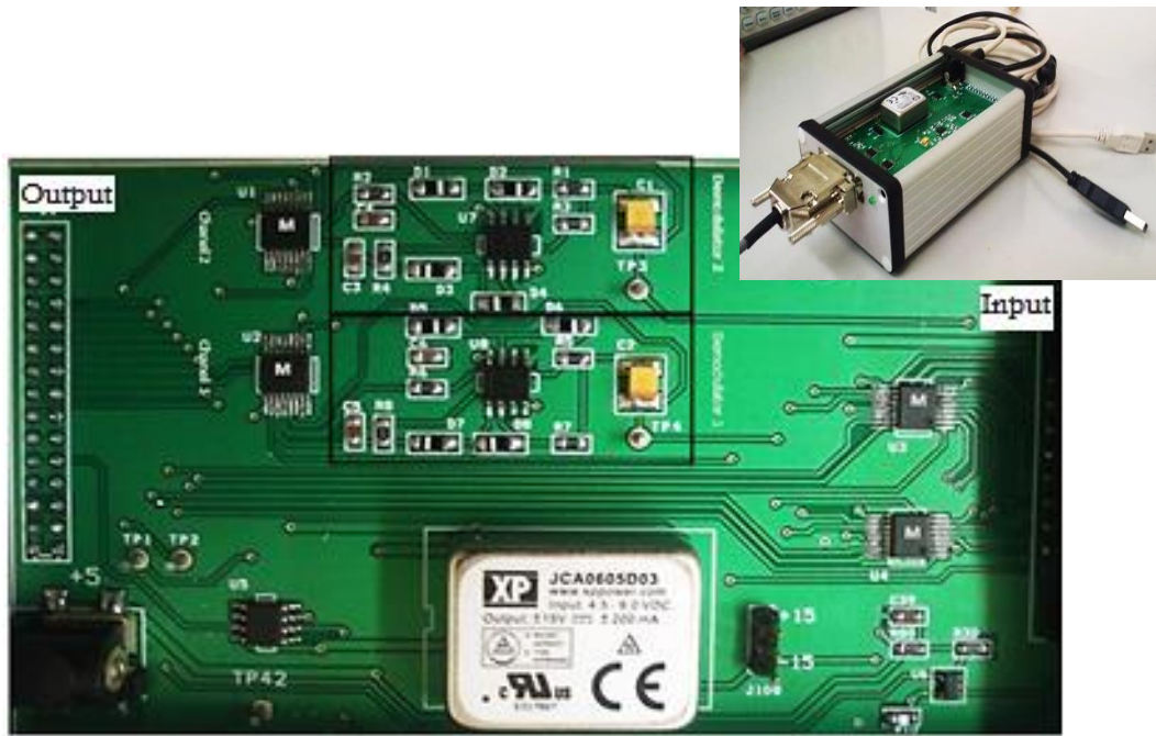
Figure 5.9: Photo of the acquisition box and the PCB containing the demodulator circuit. The acquisition box integrates not only the demodulator PCB but also the digilent. Observing the PCB it is possible to see an increase on the circuit complexity. There are two demodulator, one for each digilent channel. The electronic components marked with “M” correspond to multiplexers.
