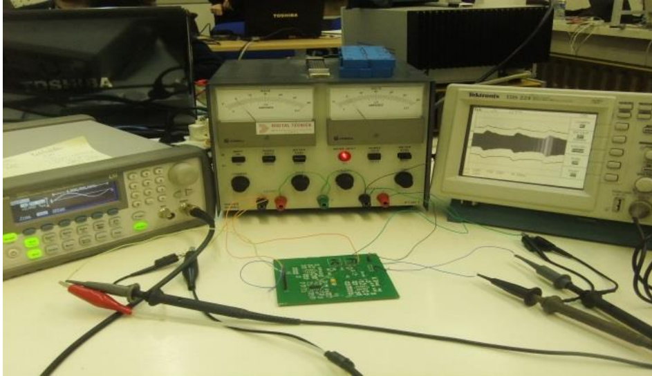
Figure 4.11: Envelope detector test on PCB. On the right, is possible to see the arbitrary waveform generator (Agilent) device which is responsible to provide the input modulated signal and, in the middle, a power source.
