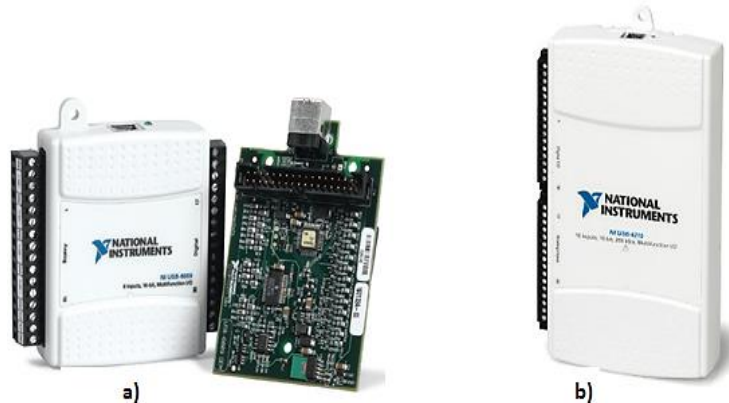
Figure 5.3: Different data acquisition devices. The image shows the two different data acquisition devices used to convert analogic to digital data. Image a) NI USB-6008; Image b) NI USB- 6210.
