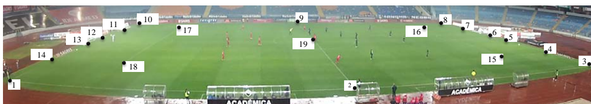
Figure 3.1. Initial calibration to extract the DLT coefficients based on real references of table 1.
