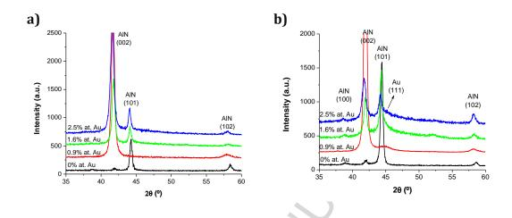
**Figure 3:** GIXRD patterns of the Al-N+Au films with different Au contents **a)** before and **b)** after thermal annealing at 400°C.
