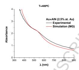
**Figure 11:** Absorbance curve of the AlN sample containing 2.5% at. Au together with the resulting simulation based on the MG approach.
