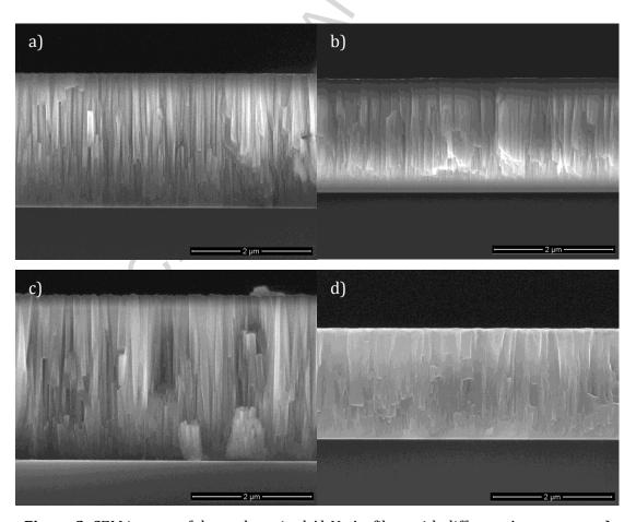
**Figure 2:** SEM images of the as deposited Al-N+Au films with different Au contents: **a)** 0% at. **b)** 1.2% at. **c)** 2.0% at. **d)** 2.5% at..
