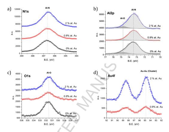
**Figure 6:** XPS spectra of the as grown Au-AlN samples concerning the **a)** N 1s **b)** Al 2p **c)** O 1s and **d)** Au 4f core levels. The experimental points are presented together with the fittings used for deconvolution (the Shirley background is not shown).
