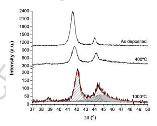
**Figure 4:** GIXRD pattern of the Al-N+Au (2.5% at. Au) sample before and after the thermal annealing treatments (at 400°C and 1000°C).
