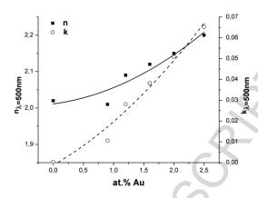
**Figure 9:** Refractive index and extinction coefficient of the Au+AlN samples with different Au contents calculated from the transmittance curves (the trend lines are just a guide for the reader).
