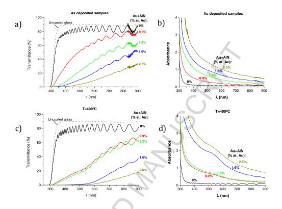
**Figure 8:** Transmittance spectra of the Au+AlN nanocomposites **a)** before and **c)** after annealing at 400°C; Absorbance spectra of the Au+AlN nanocomposites **b)** before and **d)** after annealing at 400°C.
