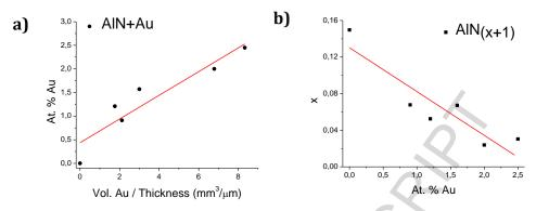
**Figure 1: a)** Volume of gold sputtered normalized to the hfilm thickness versus the atomic Au concentration determined by EPMA **b)** Deviation from the stoichiometry in the  $AlN_{1+x}$  matrix with the Au content (the trend lines are only a guide for the reader).
