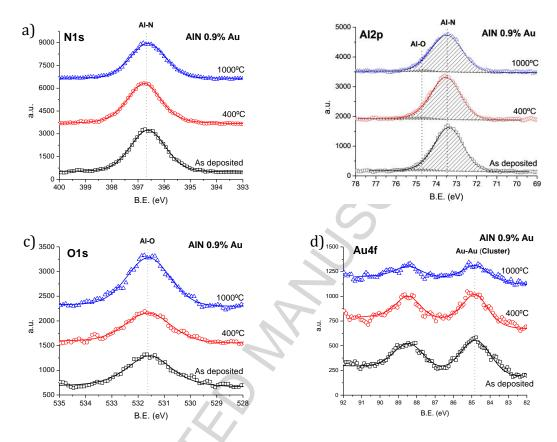
**Figure 7:** XPS spectrums of the sample containing 0.9 % at. Au before and after two different thermal treatments, concerning the core level **a)** N 1s **b)** Al 2p **c)** O 1s and **d)** Au 4f. The experimental points are presented together with the fittings used for deconvolution (the Shirley background is not showed).
