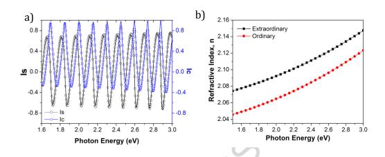
**Figure 10: a)** Fitting obtained for the pure AlN sample, where the ordinary and extraordinary refractive index of the AlN thin film were extracted as shown in **b)**.
