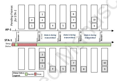
Figure 1: Legacy PSM algorithm operation example.
