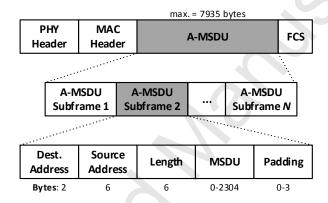
Figure 4: IEEE 802.11 A-MSDU aggregation scheme.
