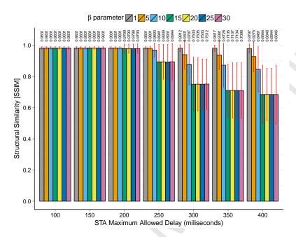
Figure 13: SSIM for distinct  $\beta$  configurations and Maximum Allowed Delay defined by the STA
