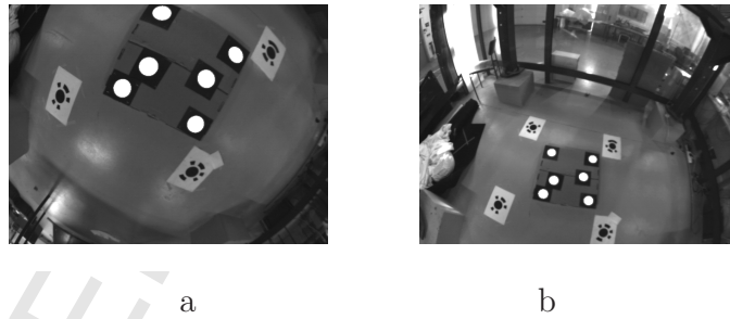
Figure 10: Initial image: a) case where only a pure rotation is considered, b) case of displacement involving translational and rotational motions
