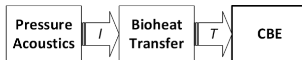
Figure 3.5: Coupling between the different models. Where I is the Intensity magnitude from pressure acoustics and T is the temperature.
