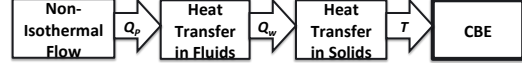
Fig. 2: Coupling between the different models. Where Q_p is the heat source from the cooper pipe, Q_w is the transferred heat from the water in the PVC chamber to the aluminum and the medium, and T is the temperature.
