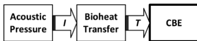
Fig. 3: Coupling between the different modules for therapeutic US heating simulation, where I is the sound wave intensity and T is the system temperature.
