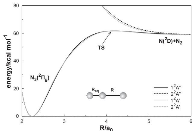
**Figure 1.** Potential energy profiles for the linear attack of a  $N(^2D)$  atom on a  $N_2$  molecule with optimized diatomic bond length. The black lines correspond to the first two  $^2A''$  states, while the gray ones to  $^2A'$ .
