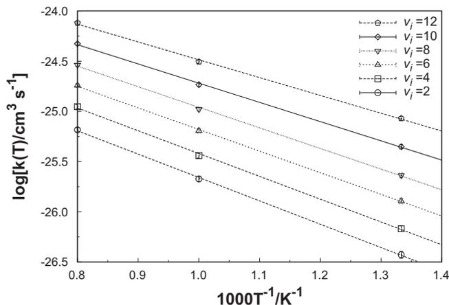
**Figure 6.** Arrhenius plot for the deactivation rate coefficients of the  $v_i \rightarrow \sum v_j < v_i$  processes.
