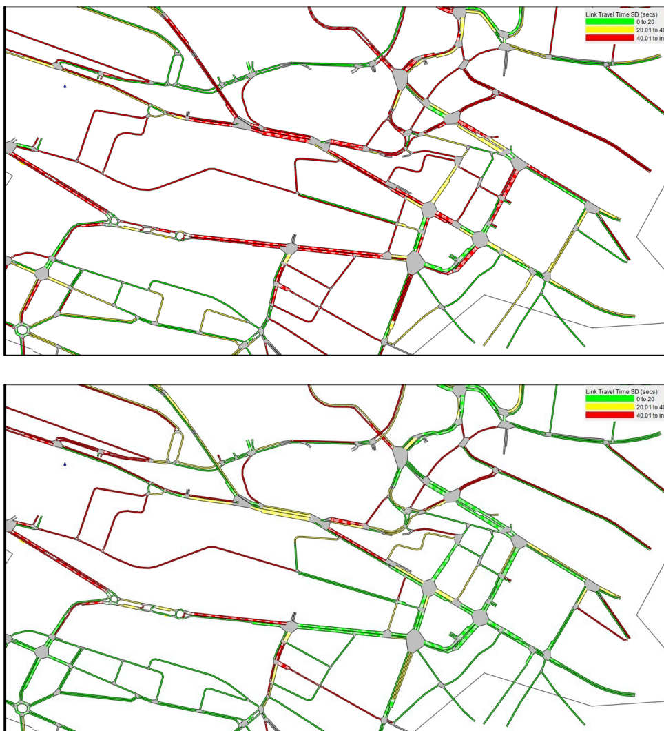
Figure 2-8: Link travel time standard deviation for initial plan (top plot) and plan obtained by solving problem P2 with metamodel m (standard deviation estimates are obtained by averaging over 50 replications).
