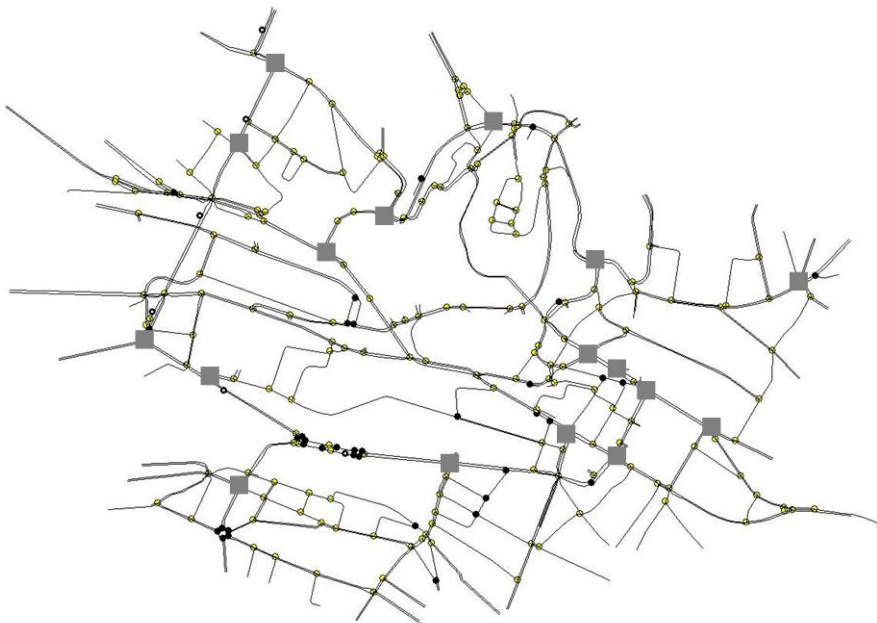
Figure 2-6: Lausanne network model with the 17 controlled intersections displayed as grey rectangles.
