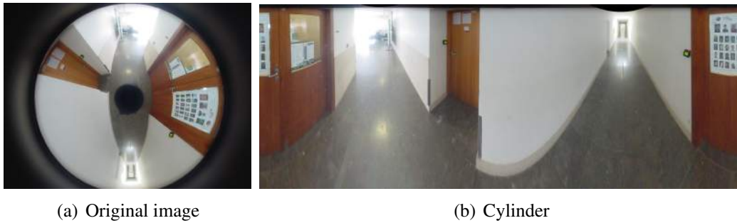
Figure 3.2: Cylindrical panorama obtained from the warping of para-catadioptric image of Figure 3.2(a).
