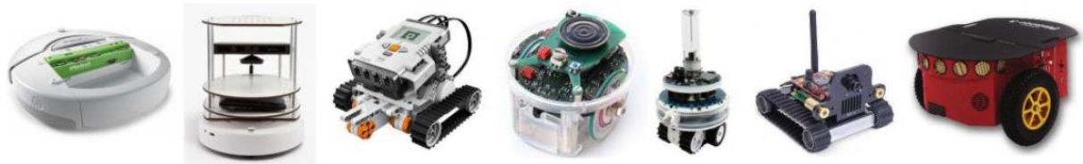
Figure 1: Some mobile robotic platforms, iRobot Create, Turtlebot, Mindstorm NXT, e-puck, MarXbot, SRV-1 Blackfin and Pioneer 3-DX.
