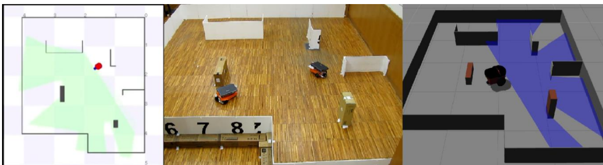
Figure 2: Robot 2D arena (Stage), real arena and 3D arena (Gazebo).
