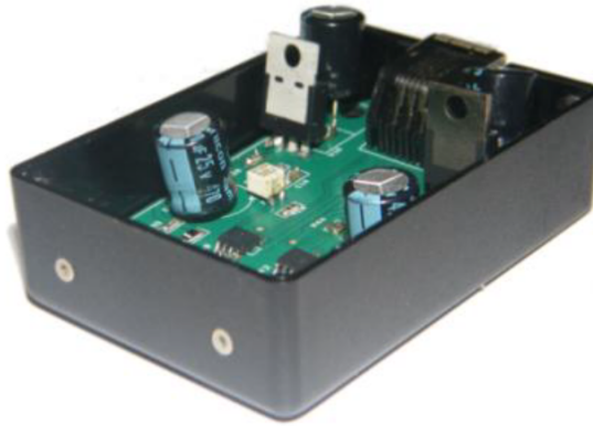
FIGURE 3.20: Photography of the laser-diode prototype.
