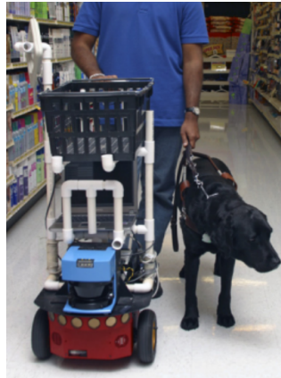
Figure 3.4: RoboCart, assistive technology to support blind people on supermarkets.[44].
