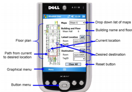
Figure 3.1: BlindAid, assisted indoor navigation system for blind people.[52].
