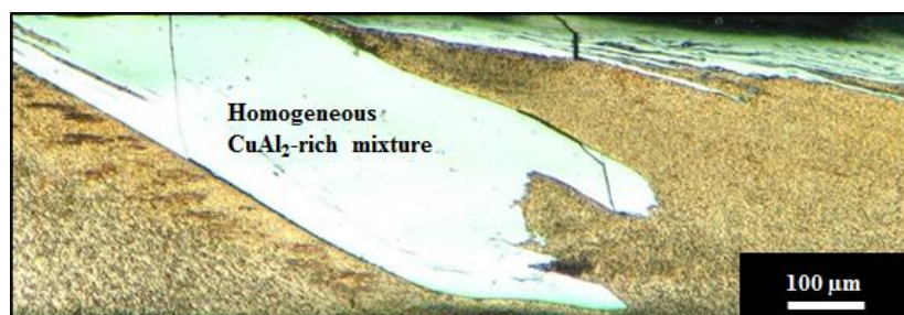
Figure 11 - Homogeneous mixture formed in the nugget of AA 5083/copper friction stir welds (adapted from Galvão et al., 2012a).
