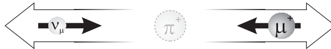
Figure 3.7: Decay of the positive pion in its rest reference frame. The emitted muonic neutrino has a definite negative helicity, implying that the positive muon's spin \vec{S}_\mu is always anti-parallel to its momentum \vec{p}_\mu .
