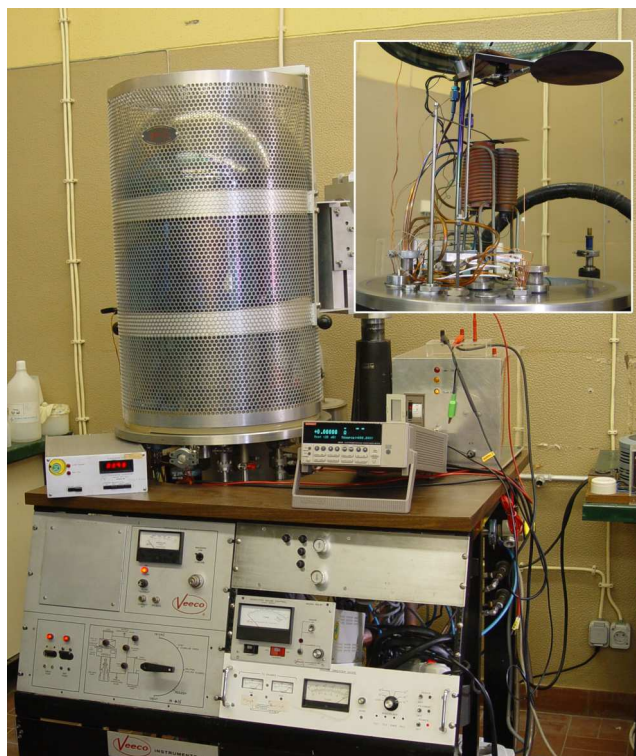
Figure 4.6: The evaporation chamber for organic thin-film deposition at the laboratory of the FNMC group in Coimbra, based in a bell-glass high-vacuum Veeco chamber driven by a diffusion pump. It possesses two resistively heated crucibles for the sublimation of organic materials, of which only one is currently connected to a power supply plus temperature controller set capable of reaching a maximum temperature of around 700 °C. The sample substrate holder may be heated up to 150 °C with a wrapped up resistive thermocoax filament connected to a low power supply source. Deposition control is performed with shutters for the ovens and sample, and the deposition rate is monitored with a quartz oscillator. The fact that a single oven power supply and a single quartz oscillator exist allows so-far the sublimation of one type of material at a time only.
