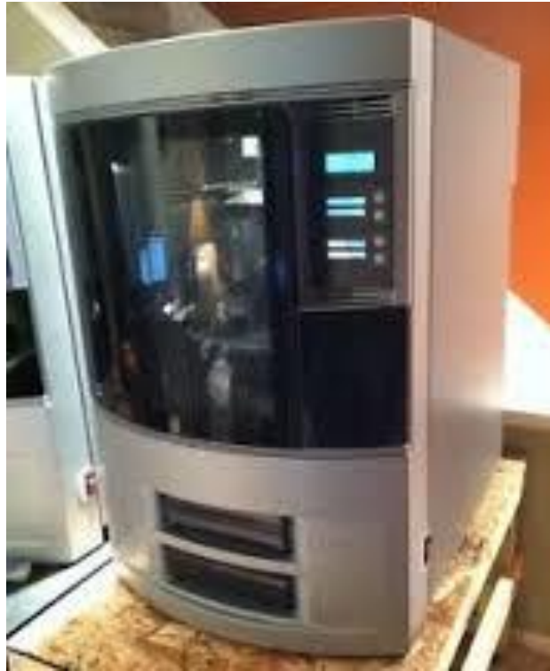
Figura 55. Impressora 3d por deposição de plástico fundido FDM, Stratasys Dimension Elite. Fonte https://encrypted-bn1.gstatic.com/images?q=tbn:ANd9GcQyB1sQhJBhaMdBEkKv3iDXJDWRT4VGLVA9EIPnbWXI9nUTM8kbA
