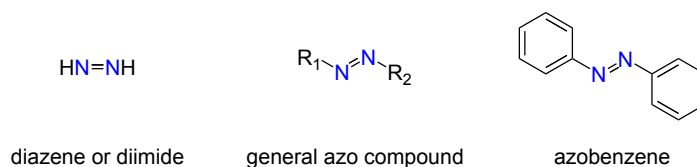
Figure 1.1 Structural formula of diimide, a general azo compound, and the most common aromatic azo compound - azobenzene. \text{R}_1 and \text{R}_2 represent hydrocarbyl groups.
