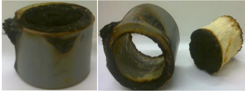
Figure 176 - Expanded Polyurethane Foam with 20 mass % of AN; horizontal position, ignited in the two surfaces.
