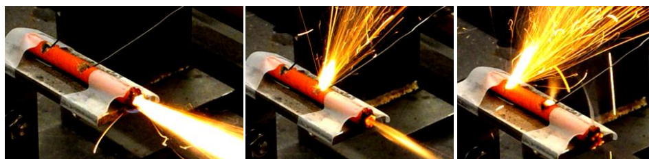
Figure 51 - Thermocouples assembly for calibration of temperature equipment and flame velocity measurement.
