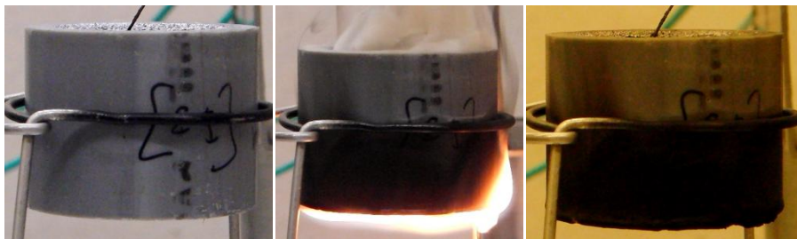
Figure 84 – Burning test of expanded PU foam with the 7 holes with cellulosic aluminium paint, horizontal position.
