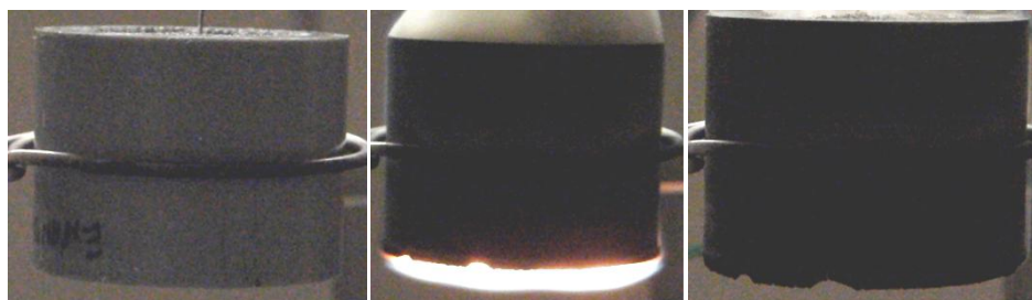
Figure 111 – Burning test of expanded PU foam with 20 mass percent of AN, with the 7 holes, painted with cellulosic aluminium paint, vertical position.
