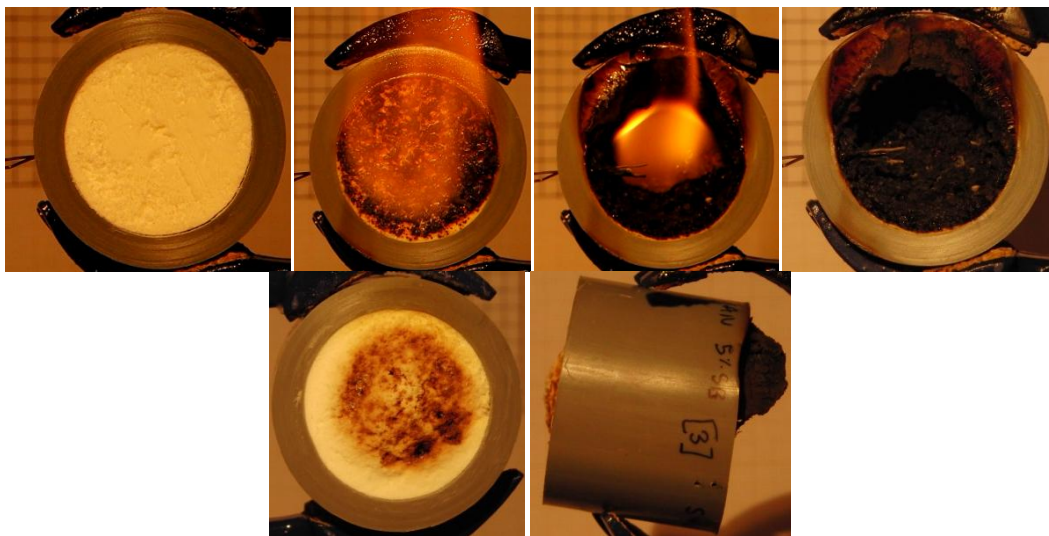
Figure 137 – Burning test of syntactic PU foam with 7 and 5 mass % of AN and SB, horizontal position.
