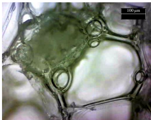
Figure 87 - Photography of microscopic investigation of expanded PU foam with 20 mass percent of AN.
