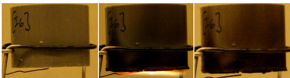
Figure 78 – Burning test of expanded PU foam, vertical position.
