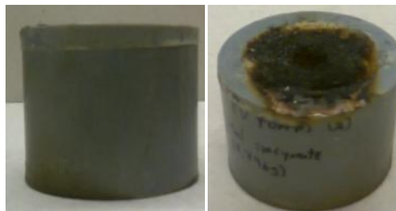
Figure 178 - Expanded Polyurethane Foam with 7 mass % of AN; vertical position, ignited in the two surfaces.
