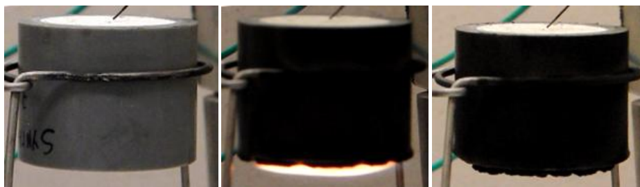
Figure 132 – Burning test of syntactic PU foam with 7 mass % of AN, painted with cellulosic aluminium paint, vertical position.
