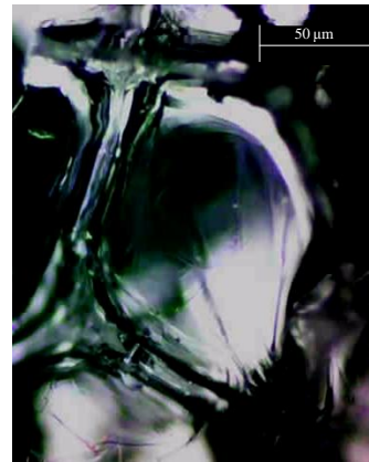
Figure 69 - Photography of microscopic investigation of expanded PU foam painted with cellulosic aluminium paint.
