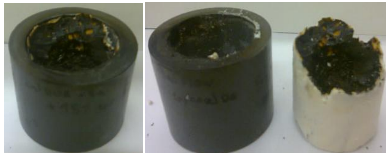
Figure 177 - Syntactic Polyurethane Foam 15%HPM; ; ignited from the top, vertical position.
