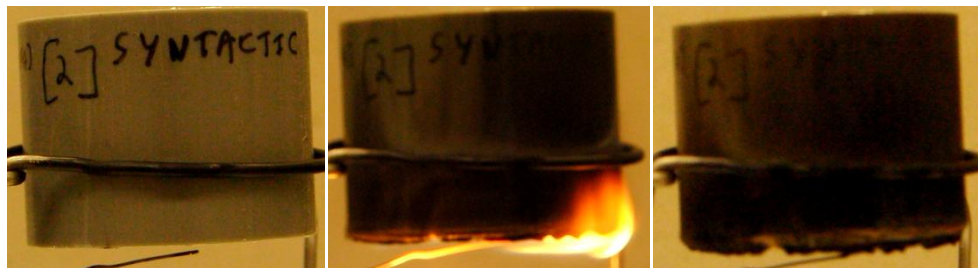
Figure 129 – Burning test of syntactic PU foam with 7 mass % of AN, vertical position.
