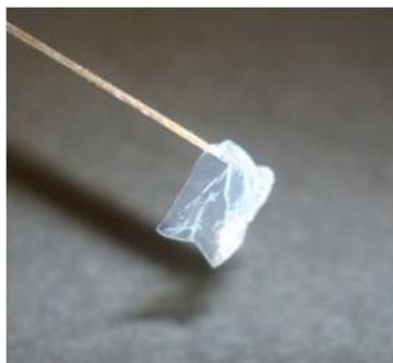
Figure 38. Visual aspect of a CBCn film loaded with 75% of [Ch][Cl] after 8 hours immersion at pH 7.
