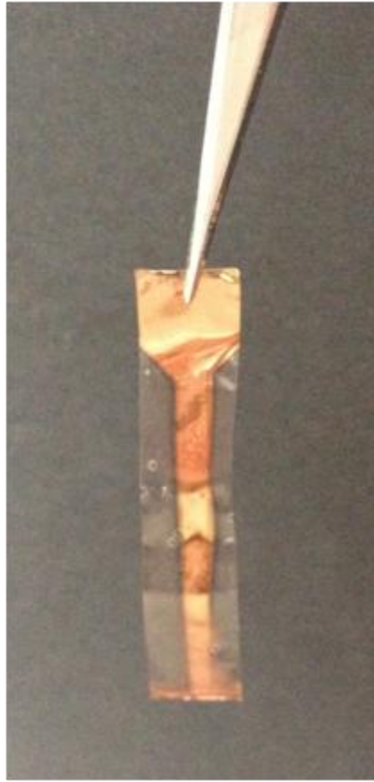
Figure 47. CS film sputter-coated with gold to study the bending angle of the films promoted by an electrical field.
