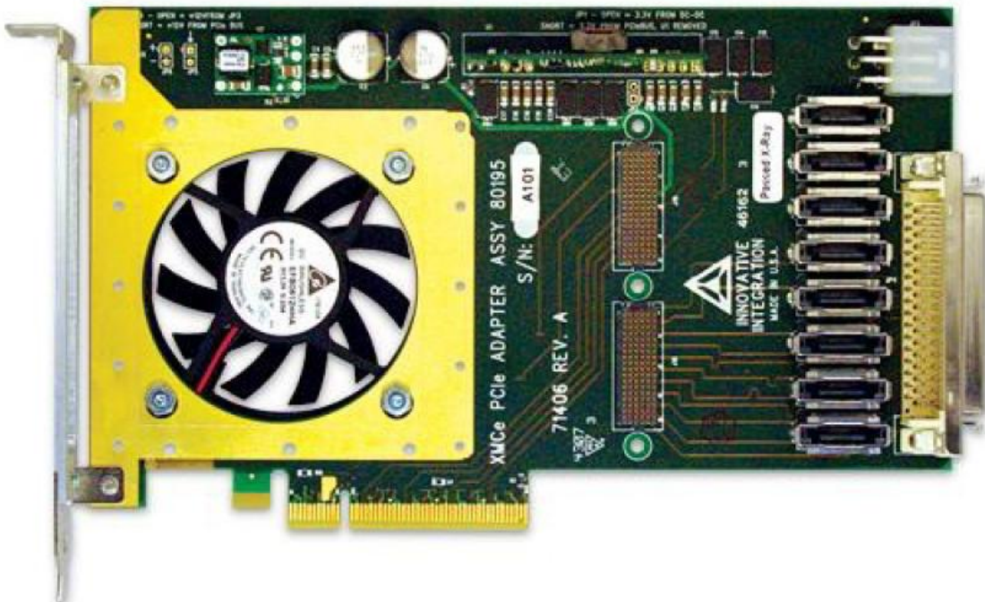
Figure 39 – Host board. Innovative x8 Lane PCI Express – XMC.3 (8x lanes) adapter card (P/N 80173-0)
