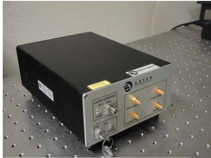
Figure 16 – Axsun Swept Source OCT bench version
