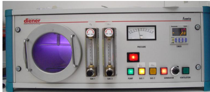
Figure 5.4 - Plasma equipment used in the surface modification of Silicone based Materials.
