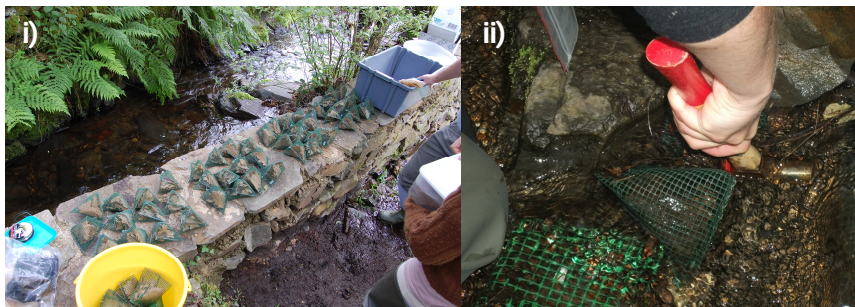
Fig. 2 Litter bags (12 × 12 cm; 4mm mesh) were prepared with ~2 g of air dried oak leaves. One A. laureatus larvae was added to half of the bags. Half of the bags were incubated at ambient and half at elevated temperature.
