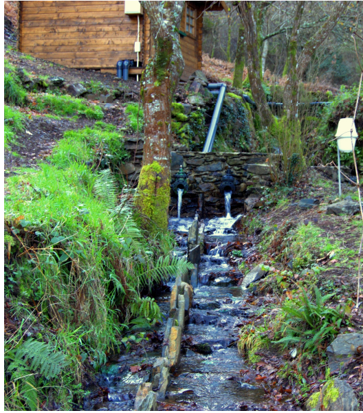
Fig. 1 Study area (Candal stream, Lousã mountain, Central Portugal 40°04'48.10''N, 8°12'11.16''W, 634 m a.s.l.). The study section was divided longitudinally along 22 m with schistose stones, each side being ~50 cm wide and 5–10 cm deep. One side of the study section was warmed up by 2.8 °C (elevated side) above the ambient temperature registered in the other side (ambient side).
