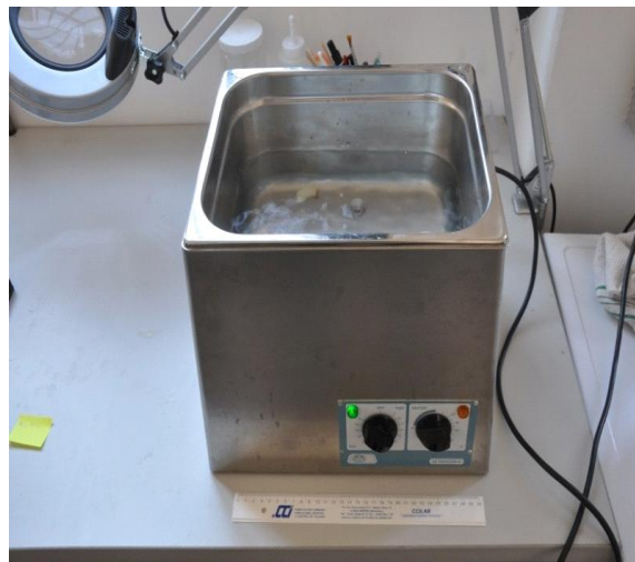
Figure 20. Suoid incisors submerged in an ultrasound cleaner with distilled water, in order to remove dust before SEM analysis.
