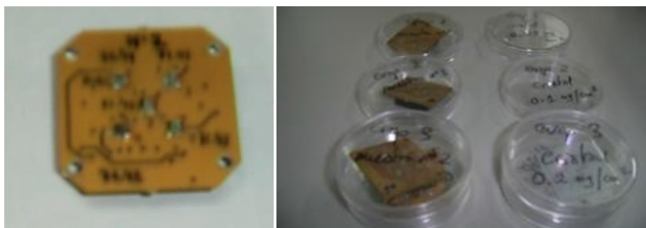
Figure 6.3. Example of a SiPM board, showing 5 Hamamatsu SiPMs (S10362 - 11 series), each one with 1\text{mm}^2 area (a); storage of several SiPM boards and coated glasses with different TPB thickness (b).
