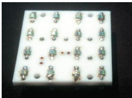
Figure 6.5. Example of a Macor SiPM board, showing 16 MPPCs of 1\text{mm}^2 .
