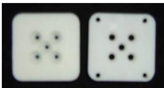
Figure 6.4. Teflon light concentrators, used for focusing the light into the 1\text{mm}^2 sensitive area of the SiPMs.
