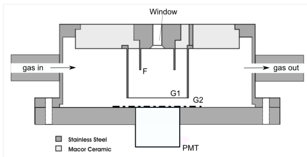
Figure 4.1. Schematic of the xenon GPSC with a R8520-06SEL PMT used as VUV photosensor.
