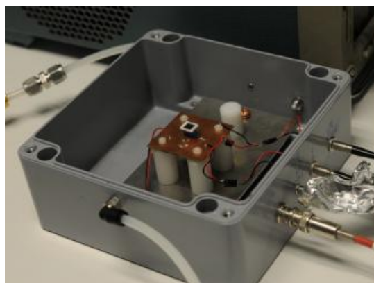
Figure A.1. Box used for the determination of the non-linearity of the APD to X-rays detection.
