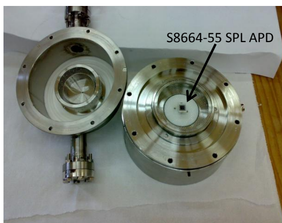
Figure 3.1. Schematics and picture of the GPSC used in this work, with the S8664-SPL APD used as VUV scintillation photosensor.
