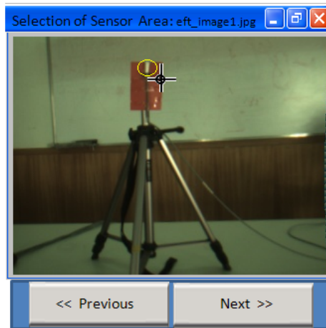
Figure C.6: Selection window: selection of the sensor region in the image to find its coordinate in the images (left and right) to allow the computation of the 3D point.
