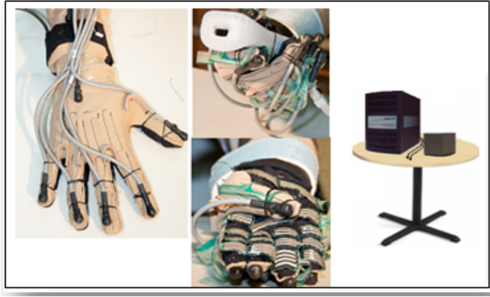
Figure 2.2: Polhemus Liberty Motion Tracking System [Pol]: Magnetic tracker sensors attached to the hand (fingertips and back of the hand).
