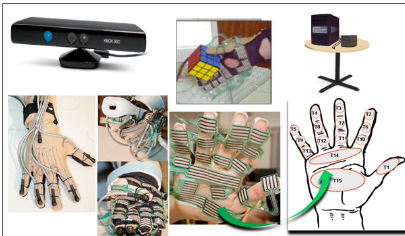
Figure 6.4: Sensors used in our experimental setup: Motion Tracking System, Tactile sensor and RGB-D sensor.
