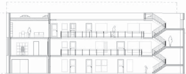
Section E, inner facade south, 1:100
